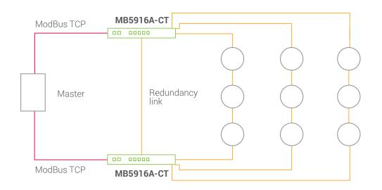
Automatic polling from serial ports with link failure recovery mechanism
