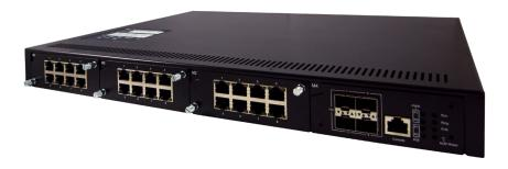
Available in *3 power input variants*, RHG7X28 is EN 61010-2-201-certified and designed to handle the harshest of environments. Its fanless design and EMC Level 3 protection guarantee operations in temperatures from -40°C to +75°C, and with 24 PoE ports running full power, it is sort the of device that can be trusted to work in your field or environment with minimum effort.
