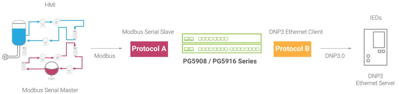
The example shows how to Easily connect a Modbus Serial HMI, through Atop's Protocol Gateway to a DNP3.0 Ethernet slave IED. The host HMI has the role of a Modbus Serial Master while the end-device to be accessed is a DNP3.0 Ethernet Server.
