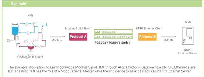
Atop's protocol Gateway acts towards the HMI seamlessly as a Modbus Serial Slave, answering the poll commands or the write commands required by the Host by its virtual Modbus ID. Meanwhile, it acts as a DNP3.0 Ethernet Client with regard to the end-device whose DNP3.0 address is mapped to the virtual Modbus ID that the HMI is accessing.
