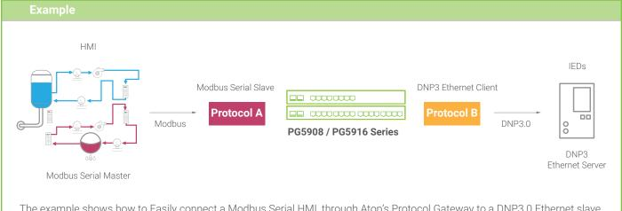
The example shows how to Easily connect a Modbus Serial HMI, through Atop's Protocol Gateway to a DNP3.0 Ethernet slave IED. The host HMI has the role of a Modbus Serial Master while the end-device to be accessed is a DNP3.0 Ethernet Server.
