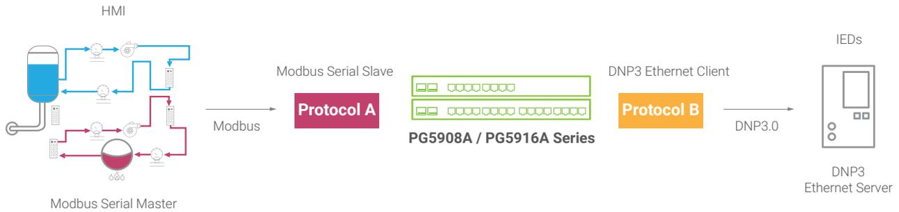
The example shows how to Easily connect a Modbus Serial HMI, through Atop's Protocol Gateway to a DNP3.0 Ethernet Server IED. The host HMI has the role of a Modbus Serial Master while the end-device to be accessed is a DNP3.0 Ethernet Server.
