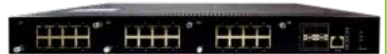
24 port Layer-2 Managed Switch, with 8 Gigabit PoE ports, 8 Gigabit RJ45 ports, 8 100/1000 SFP slots and 4 x 1/10 GbE SFP uplink slots
