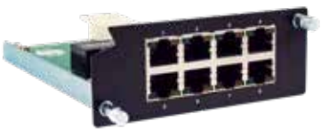
RHG7X28-M2 8-port Gigabit RJ45 module
