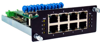
RHG7X28-M1 8-port Gigabit RJ45 PoE module
