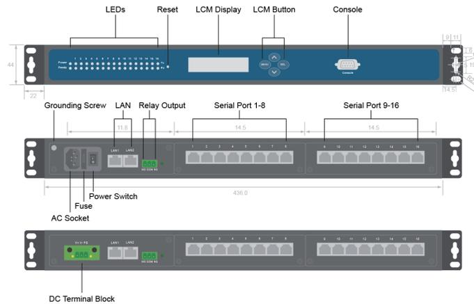
\*SE/MB/PG5908A has its serial ports 9-16 covered up compared to SE/MB/PG5916
