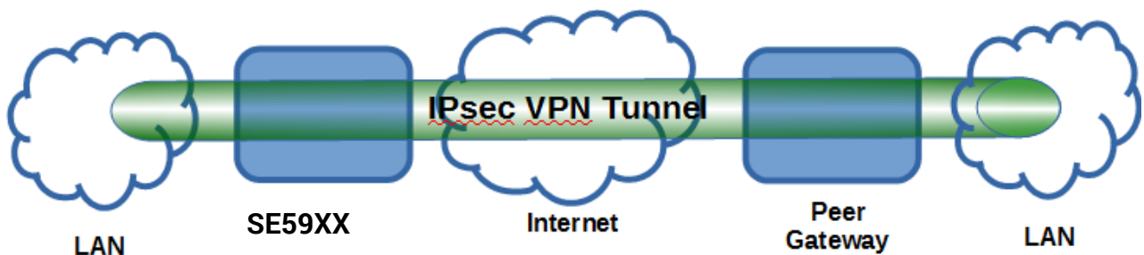
Figure 4.37 An example of network application using a subnet-to-subnet connection via the SE59XX and a peer device
