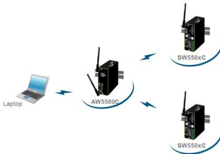
Figure 2.1 An Application of Wireless Serial Device Server in WLAN
