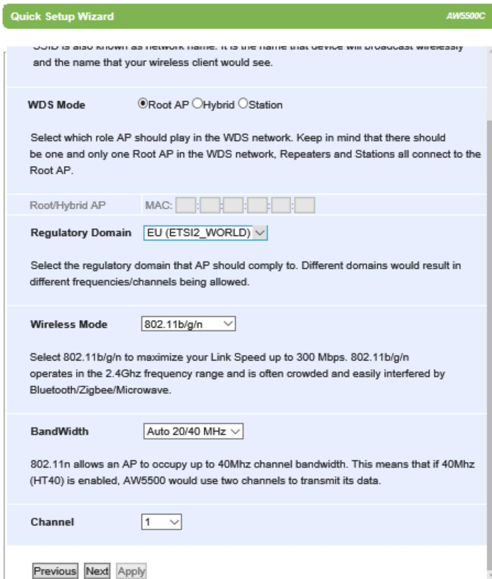
Figure 4.22 Second Wizard Web Page for WDS Bridge Operation Mode (Lower Part)
