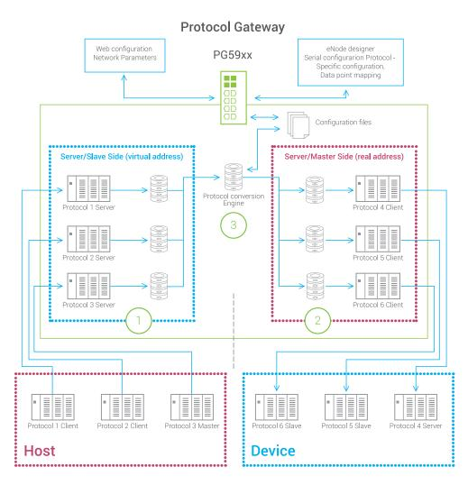
The figure below shows the device as part of a general architecture.
