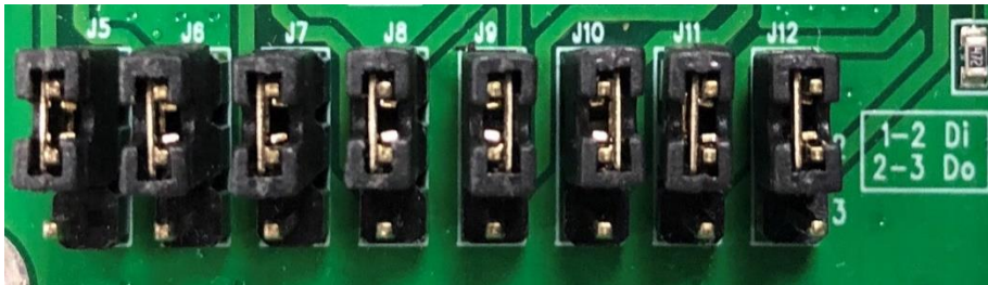
Figure 4.10 - DIO (Digital Input/Output) Jumper Settings
