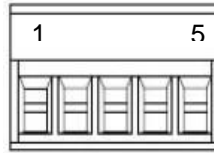
Figure 4.5 - Serial Port on TB5 (5-Pin 3.81mm Terminal Block) with Pin Assignments
