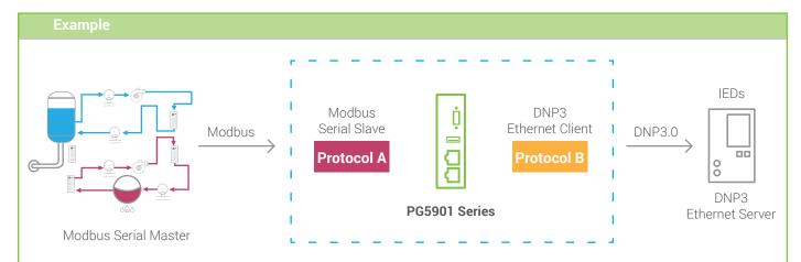
The example shows how to Easily connect a Modbus Serial HMI, through Atop's Protocol Gateway to a DNP3.0 Ethernet Server IED. The host HMI has the role of a Modbus Serial Master while the end-device to be accessed is a DNP3.0 Ethernet Server.
