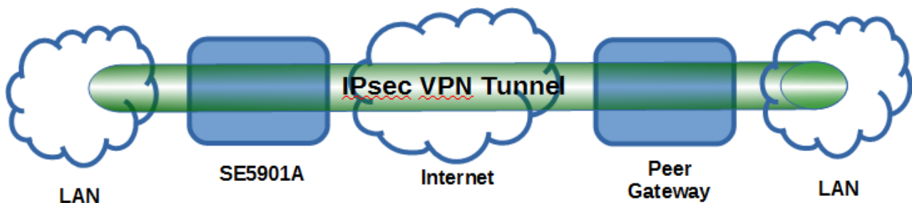
Figure 3-21 An example of network application using a subnet-to-subnet connection via the SE59XX and a peer device
