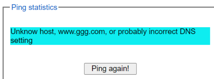
Figure 2.30 Example of unsuccessful ping command result
