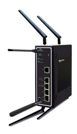
Besides mesh, the device can still do the legacy functions such as standard AP or STA (client). With optional PoE power or additional Serial ports, the device is also available as a Serial Server / Protocol Gateway / Modbus Gateway.
