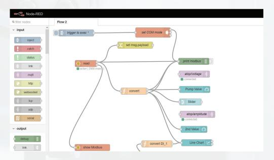
Node-RED's dashboard nodes provide a comprehensive set of UI components for building fully functional dashboards that are suitable for IIoT and industrial applications. Known as Dashboard Widgets, they include bar charts, donut charts, gauges, notifications, basic text, as well as sliders, inputs, and forms.
