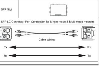
The SFP slot should be used in conjunction with a MSA compliant optical transceiver
