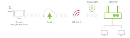
CR5201B is also designed to act as a cyber security gateway. Un-secured network access will be denied by the firewall protection, while secured VPN tunnels enhance the security of your data transmission during the network communication. Security and encryption are indispensable to IoT, and therefore fundamental functions of CR5201B.
