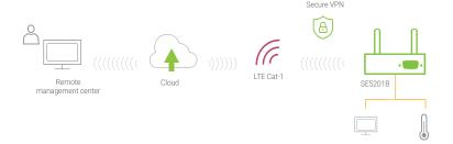
SE5201B is also designed to act as a cyber security gateway. Un-secured network access will be denied by the firewall protection, while secured VPN tunnels enhance the security of your data transmission during the network communication. Security and encryption are indispensable to IoT, and therefore fundamental functions of SE5201B.
