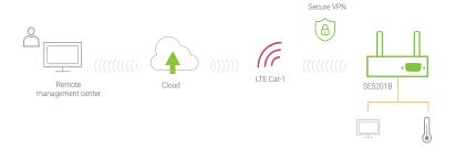
SE5201B is also designed to act as a cyber security gateway. Un-secured network access will be denied by the firewall protection, while secured VPN tunnels enhance the security of your data transmission during the network communication. Security and encryption are indispensable to IoT, and therefore fundamental functions of SE5201B.
