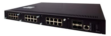
Available in **3** power input variants, RHG7X28 is UL/EN62368 certified by specifying the complete safety requirements for control equipment and designed to handle the harshest of environments. Its fanless design and EMC Level 3 protection guarantees operations in wide temperatures from -40°C to +75°C, and with 24 PoE ports running full power, it is a device that can be trusted to work in your field or environment with minimum effort.
