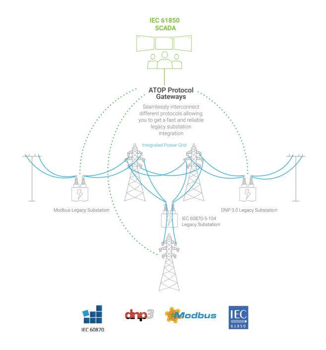
The pivotal role of protocol gateways lies in their ability to act as translators, allowing devices from different eras and communication paradigms to understand each other. Specifically, this involves the translation of data points, mapping of attributes, and normalization of data formats to ensure a coherent and standardized communication flow. Architecture of a protocol gateway consists of three parts:
