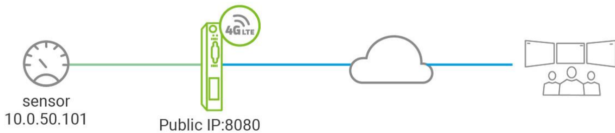
Figure 4-22 Example of Port Forwarding through PG5201B Low-Power Protocol Gateway
